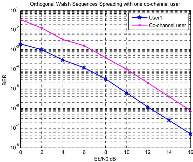
Figure (2): Number of paths 3 User1 delays 0; 2; 6 samples and co-channel user paths delays 0; 3; 6 samples
