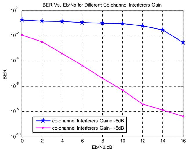
Figure (3): BER vs. Eb / N0 of the desired user for different values of Co-channel interferer's power gain (-6,-8dB)
