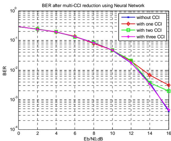
Figure (11): BER performance after multi-CCI reduction using neural network
