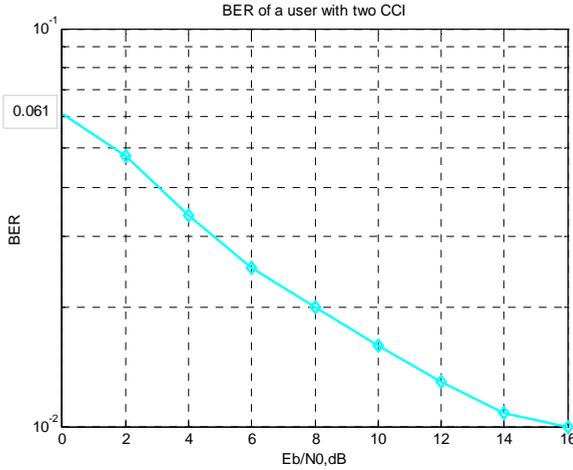
Figure (5): A single user interfered with two co-channel interferers
