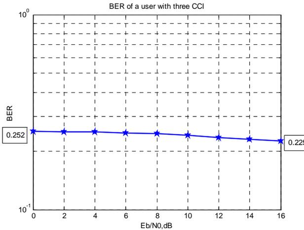
Figure (6): A single user interfered with three co-channel interferers
