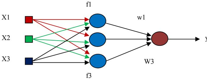
Figure (7) Radial basis neural network architecture
