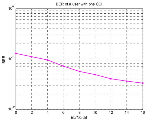
Figure (4): Number of paths 3 User1 with paths delays 0; 2; 6 samples, co-channel user with paths delays 0; 3; 6 samples and interferer's gain -6dB
