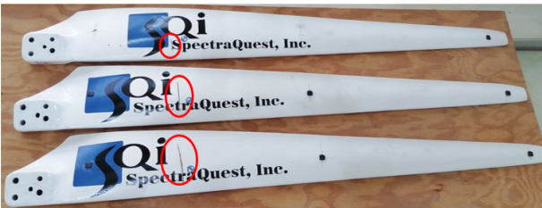
Figure 5: Three transversely defective blades (three crack levels)
