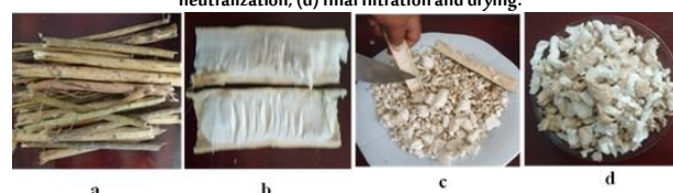
Figure 2. Stepwise NaOCl-based extraction process of sunflower stem pith (Ahmed, et al. , 2025) (a) Initial water and NaOCl soaking, (b) NaOCl-only treatment, (c) rinsing and neutralization, (d) final filtration and drying.
