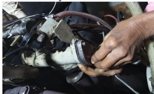
Figure 4. Air manifold seal
