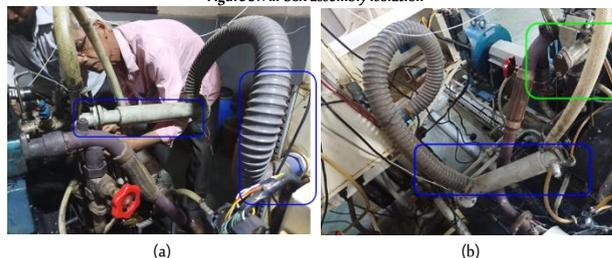
(a) Air box is connected to the engine intake manifold
